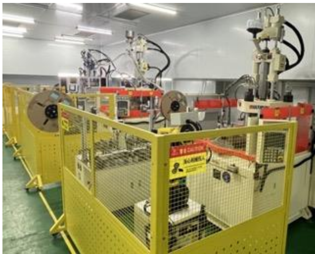
汽车雷达产品机械手臂自动上料 Automatic feeding of robotic arms for automotive radar products
